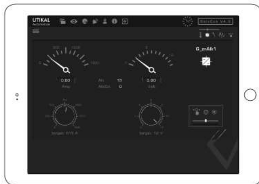
Components such as temperatures, rectifiers, dosing pumps, various switches and other details are called up and displayed separately as required.
