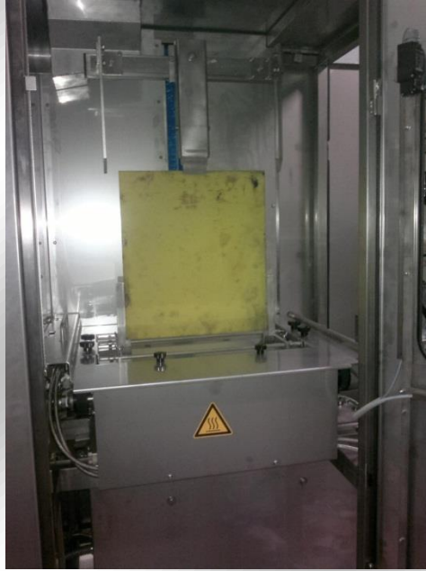
Covers easy to remove for maintenance
