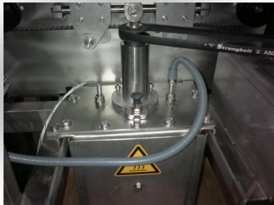
Easy access to the removable solder pump
