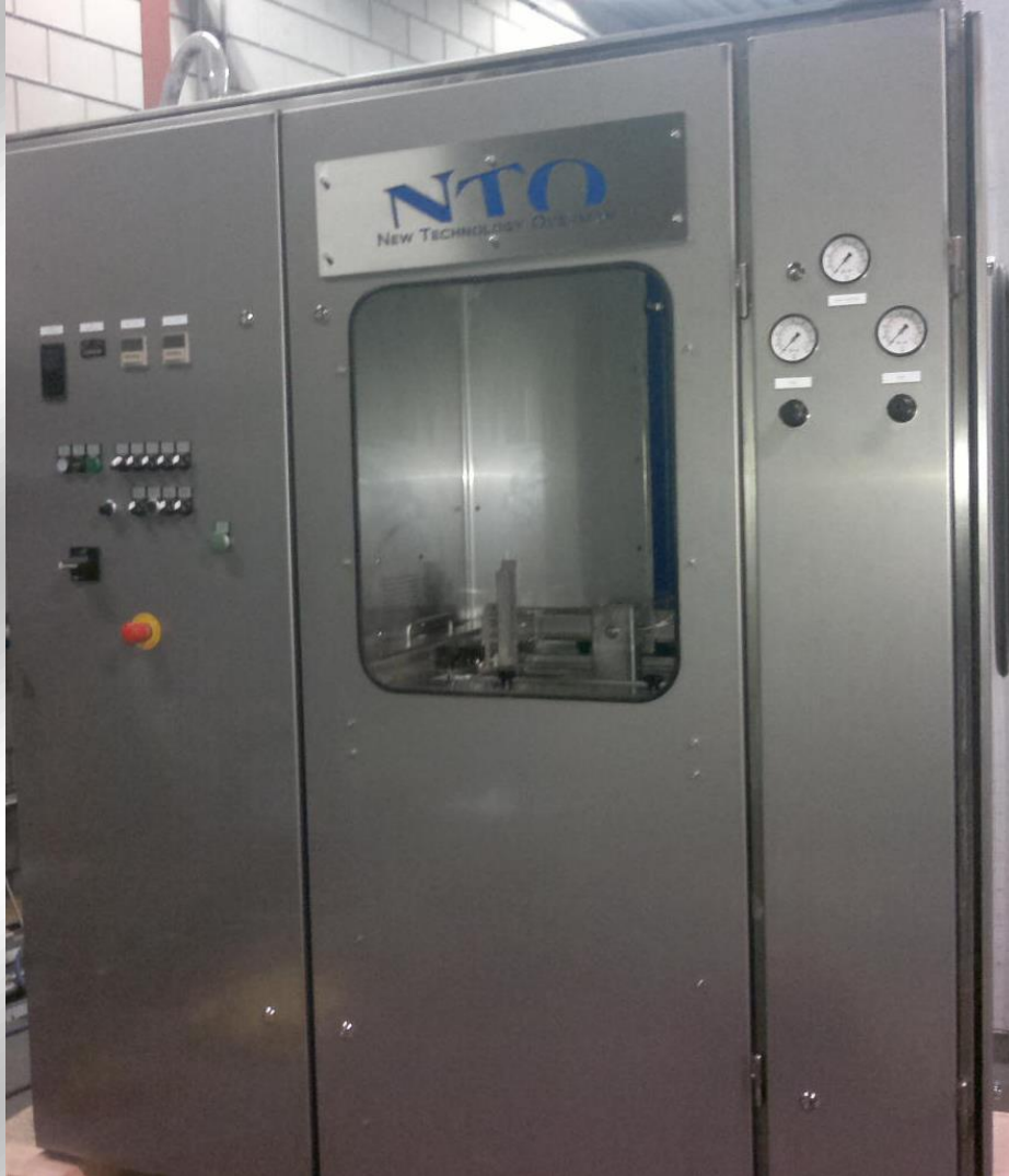
Stainless steel covers, Electrical cabinet and Pneumatic cabinet
