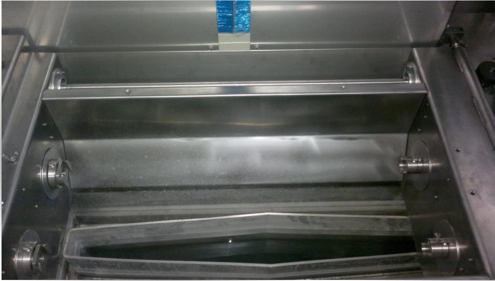
Solder pot made of Stainless steel 316L material. Air knives easy removable.
